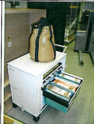
picture 3: unit strength test Concentrated functional load
