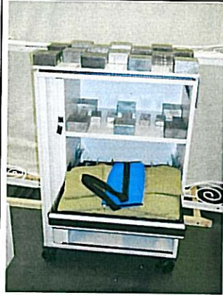
picture 1: unit strength test Distributed functional load
