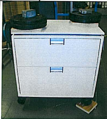
picture 5: racking resistance test
