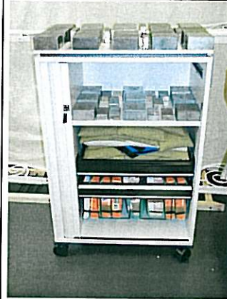
picture 2: unit strength test Distributed proof load
