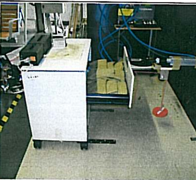
picture 7: extendible element out- stop test
