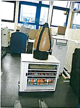
picture 4: unit strength test Concentrated proof load
